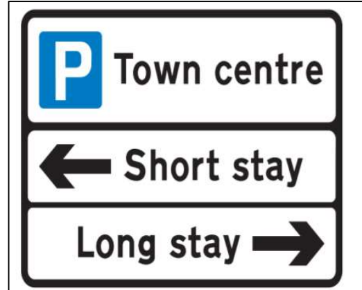
Figure 34: Directional Car park Sign Example
